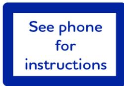
When a consumer device indicates to the reader that consumer interaction is required, the contactless-enabled ATM shall display the “See phone for instructions” message (as specified in *EMV Contactless Specifications for Payment Systems*) and power down the contactless interface.
